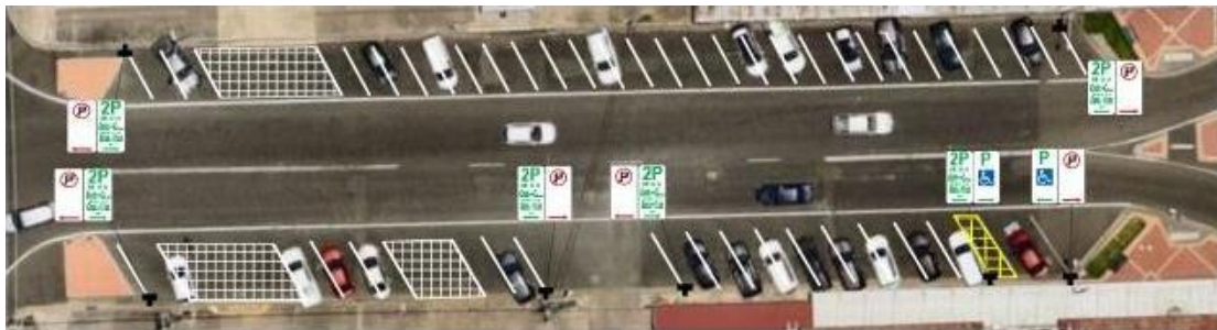
Figure 4 – Proposed car park marking on Bourke Street (between Kable Avenue and Peel Street)
