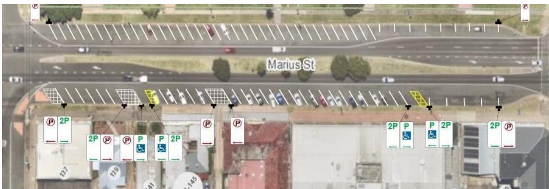
Figure 2 – Proposed car park marking on Marius Street (between Bourke Street and Brisbane Street)
